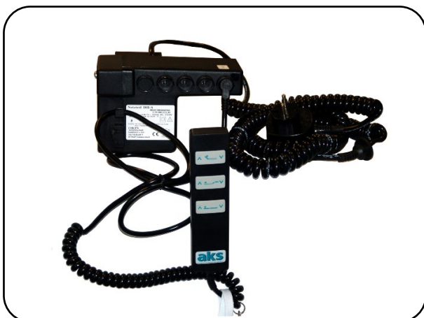
Fig. 4.11 – Mains adapter with integrated controller, mains plug incl. mains power cut-off and manual control unit incl. lock key
