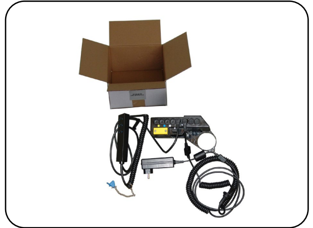
Fig. 4.08 – Controller, mains adapter (SMPS), manual control unit including lock key
