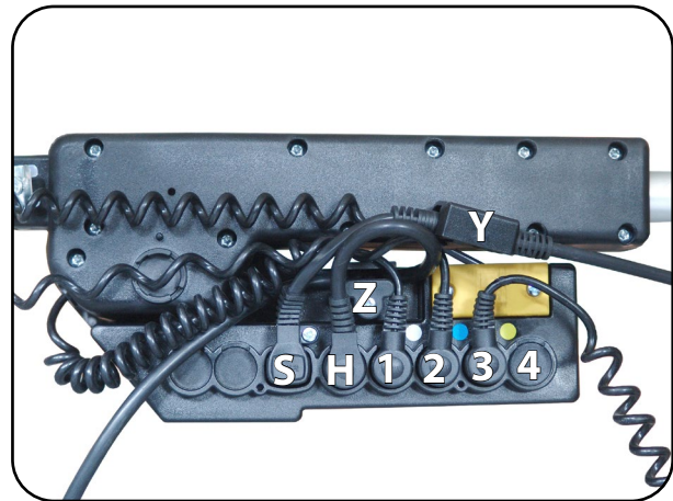
Fig. 6.2.05 – Controller with motor power cables
