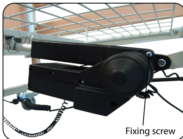
Fig. 6.2.03 – Controller on back part drive
