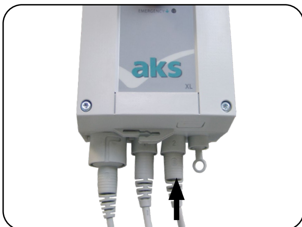
Fig. 6.2.05 - Connect spreader drive
