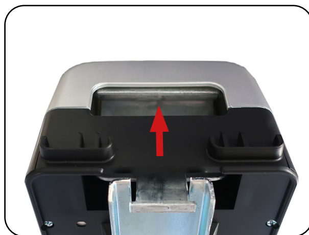
Fig. 8.7.02 – Unlocking lever on the battery pack
