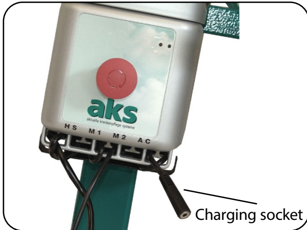
Fig. 8.7.05 – Control unit with charging socket
