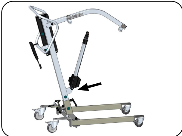
Fig.13.2.01 – Dismantling the lift drive
