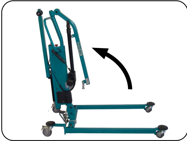
Fig. 6.2.03 – Setting up the stand mast
