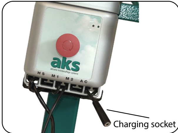
Fig. 8.7.05 – Control unit with charging socket
