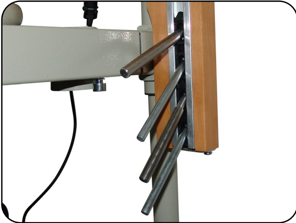
Fig. 6.4.03 – Side bar sliders in the aluminium rail
