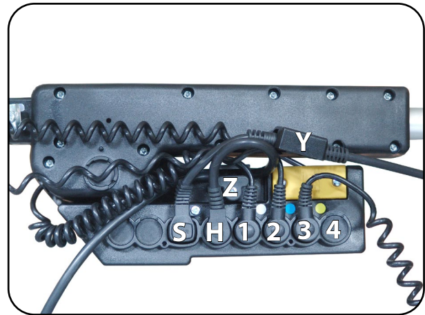
Fig. 6.2.05 – Controller with motor power cables
