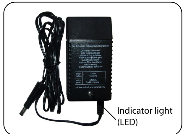
Fig. 8.7.06 – Charger with power supply line
