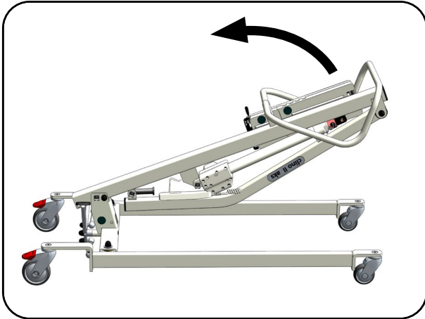
Fig. 6.2.03 – Setting up the stand mast
