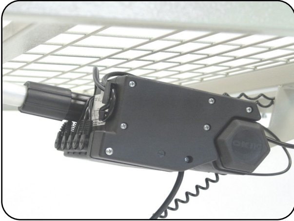
Fig. 6.2.01 – Controller on back part drive
